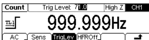
Figure 2-63 To set the coupling mode
