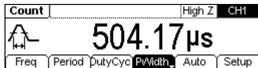
Figure 3-28 Positive Width View
