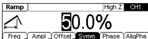
Figure 2-10 Ramp Signal Parameter Setting Interface
