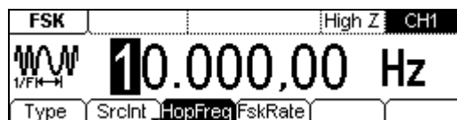
Figure 2-39 FSK Waveform Parameter Setting Interface
