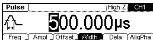
Figure 2-13 Pulse Signal Parameter Setting Interface
