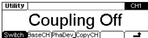
Figure 2-60 Channel Coupling Setting Interface
