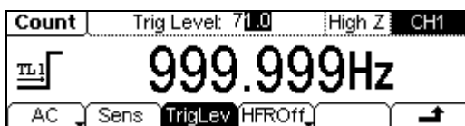
Figure 2-66 To set the high frequency restrain on/off
