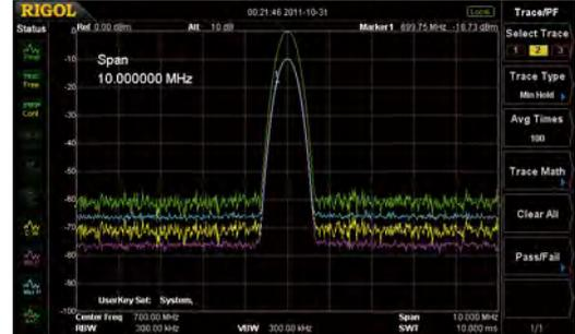
Zero span to demodulate the AM signal
